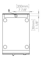
NOTES: A- WATER DRAIN, 1.2" O.D. B- ELECTRIC CONNETOR, 220V 1PH 60Hz
