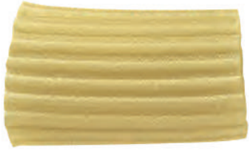
#83 26.5 mm new [1.4 mm wall thickness] [with ridges]
