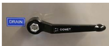
Horizontal = Drain Closed
