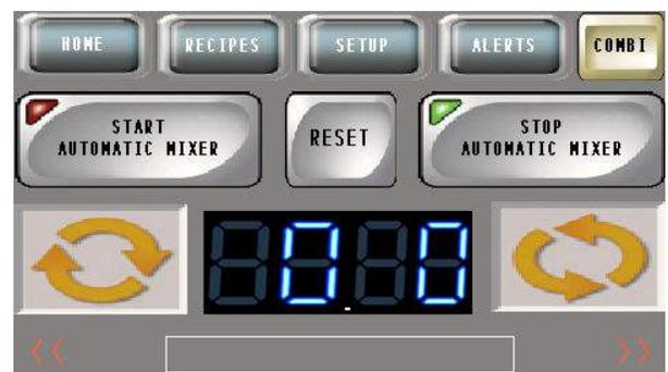
**WARNING:** If the mixing/kneading tank runs and the mixing shaft turns in the opposite direction of the signal on the display, it is necessary to invert the two feeding phases.
