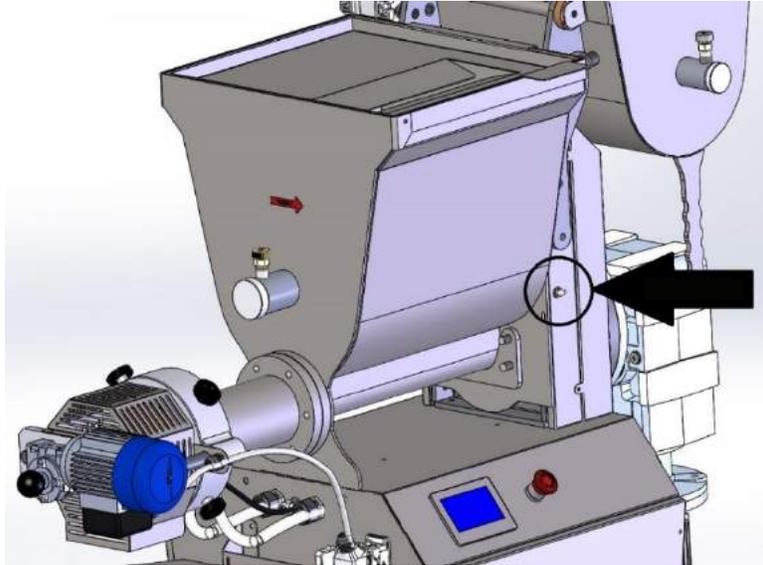
The grease replacement operation is complete when clean grease comes out from the exhaust fitting:
